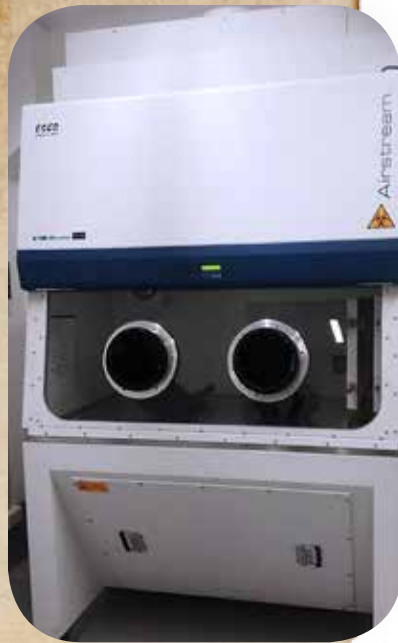
Airstream® Class III Biological Safety Cabinet Recipient of IAEA Technical Cooperation Project Dr. Jose N Rodriguez Memorial Hospital PHILIPPINES
