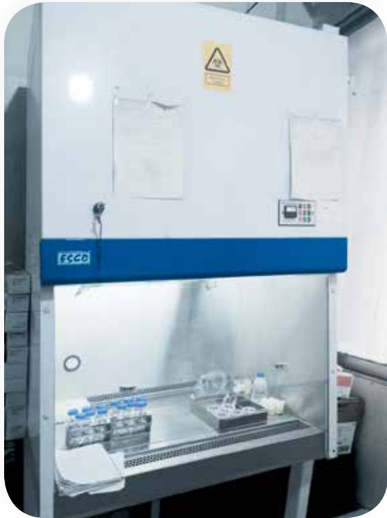
18 year-old Biological Safety Cabinet BIRDEM General Hospital BANGLADESH
